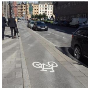
2. Bicycle paths on the sidewalk, delimited only by the pavement and by the parking spaces at the curb.
